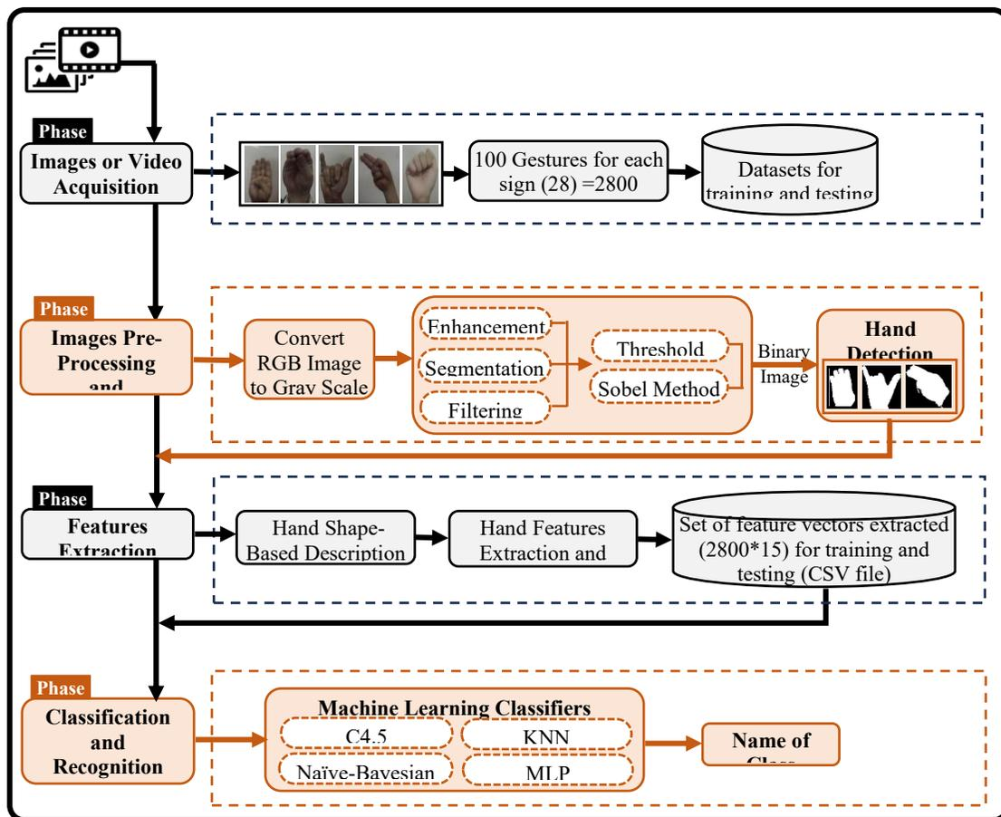
**Figure 1: Major phases of the alphabet based ArSL recognition system**
